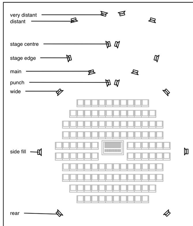
**Figure 1: Duplication of stereo pairs in BEAST diffusion system (adapted from Harrison 1998: 19)**
